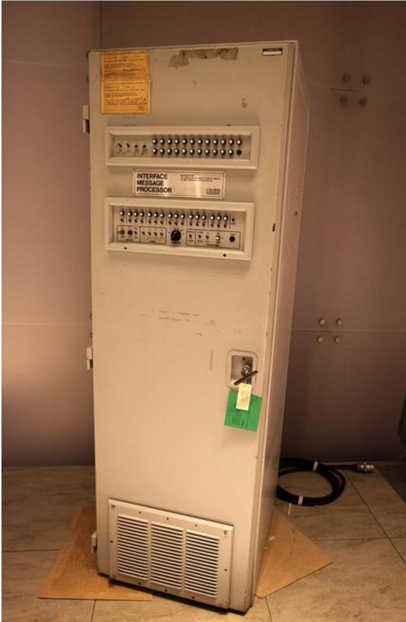
An internet router, circa 1965: a wardrobe-sized Interface Message Processor, or IMP, modified by Bolt, Beranek and Newman from a Honeywell DDP-516 'minicomputer'. Each node in the fledgling ARPANET consisted of an IMP. (Image courtesy of [Jurvetson on Flickr](#).)
